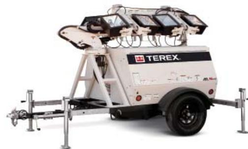
**With over 28 ft (8.5 m) of vertical height and 20 ft (6.1 m) of horizontal outreach, the Terex AL5 HT is perfect for mining industry applications.**
