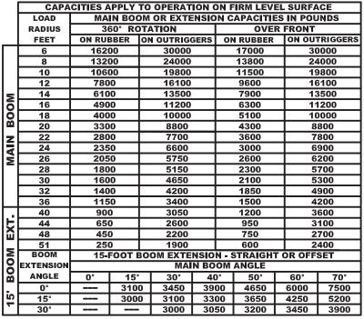
LOAD RADIUS IS THE HORIZONTAL DISTANCE FROM THE CENTER OF ROTATION OF THE UNLOADED CRANE TO THE VERTICAL LOAD LINE WITH THE LOAD APPLIED.
