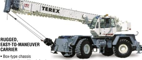
Box-type chassis construction with reinforcing cross members.
